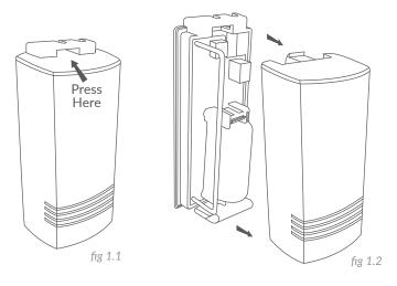
**STEP 1**Applying pressure near the sensor's locking tab(fig 1.1), remove cover by pulling away from the base(fig 1.2).
